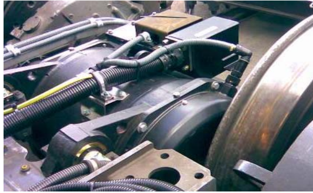
Figure 4: The MITRAC PM motor mounted in the REGINA test train bogie.
