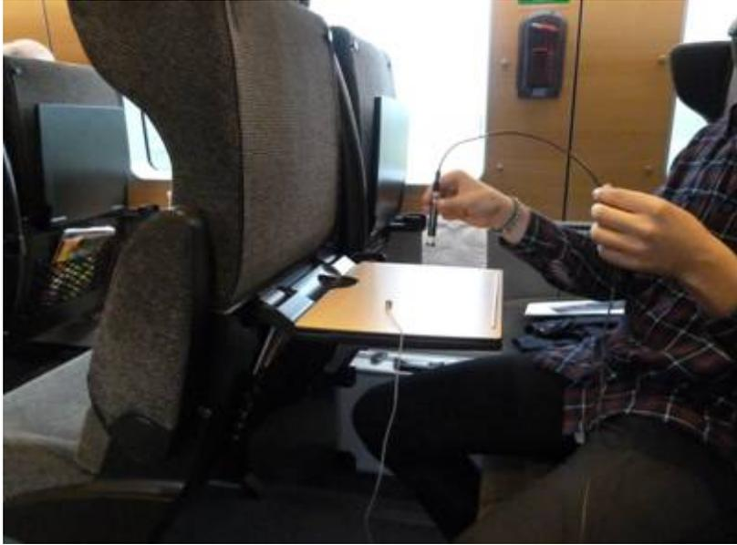
**Figure 14** Sound and acceleration measured on table mounted on seat. Seat in front free.
