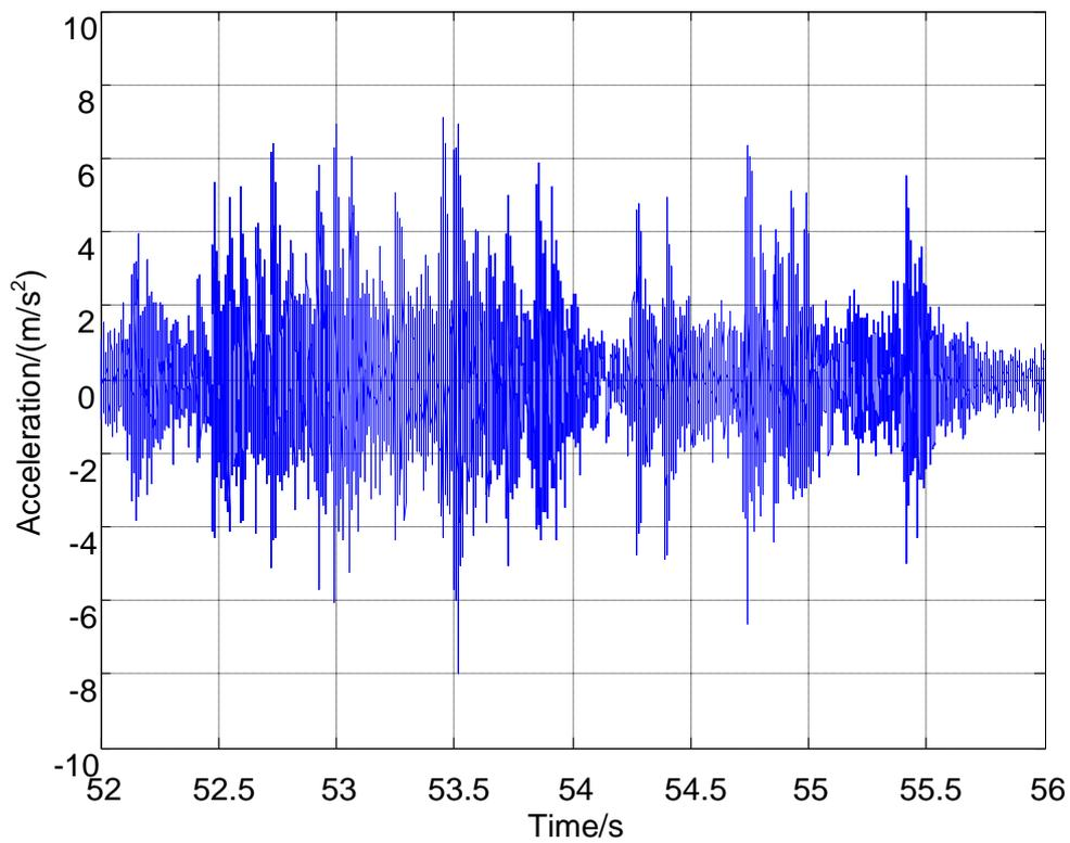
**Figure 7** Acceleration signal measured on rattling light cover. Note the impacts appearing with roughly 0,1 s time interval and the long reverberation time. This sound is rattling with a metallic sound.
