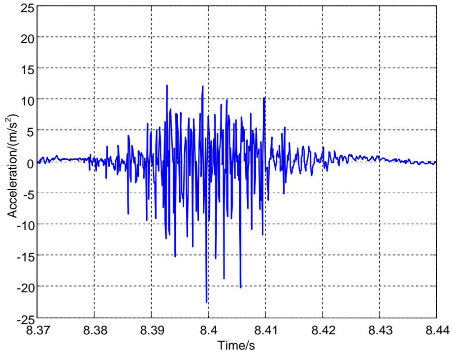
**Figure 11** Acceleration signal measured on scratching light cover. Note that the acceleration starts at a low value the sticks and slips with increasing amplitude and finally gradually decays to a low value.
