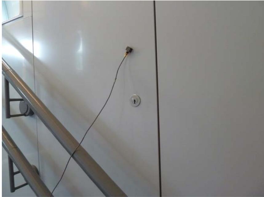
**Figure 2** Accelerometer placed on cabinet door. Strong bursts of vibration are excited when the door impacts the door frame.
