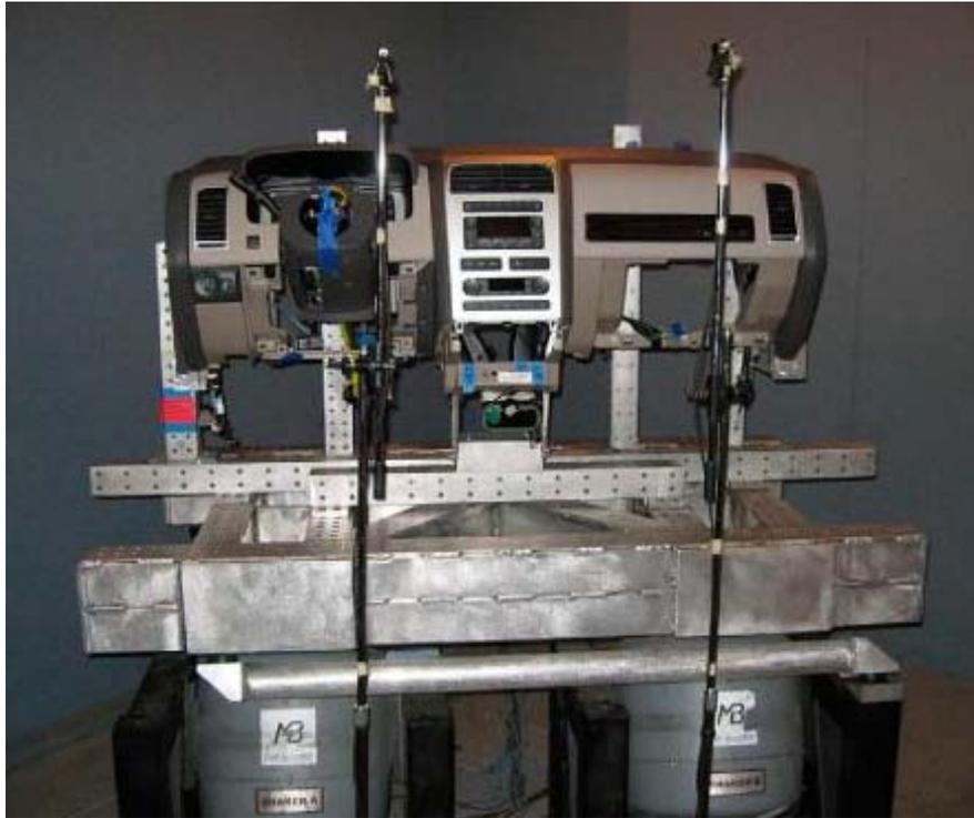
**Figure 21** Component testing in environmental test bench. From reference [16 Martin Trapp, Ford Motor Company, Text book].
