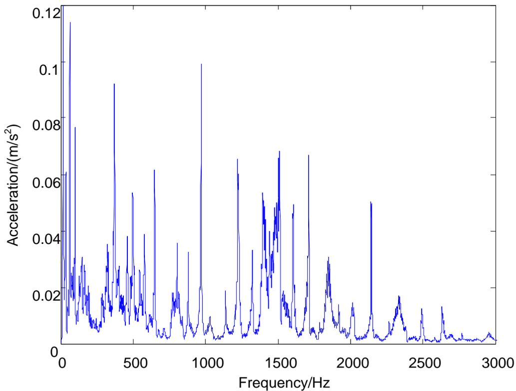
**Figure 8** Acceleration spectrum measured on rattling light cover.
