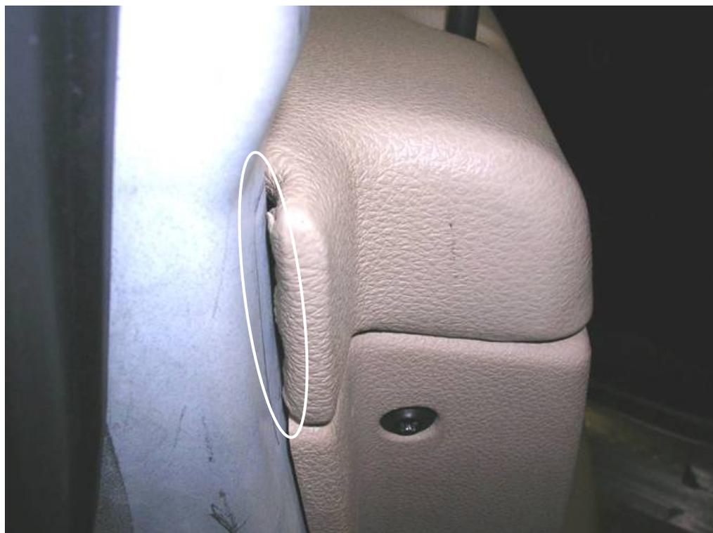
**Figure 20** Example: Add Flock tape (or increase retention) to prevent vinyl to sheet metal squeak. From reference [23 Martin Trapp, Ford Motor Company, 5-18-06]
